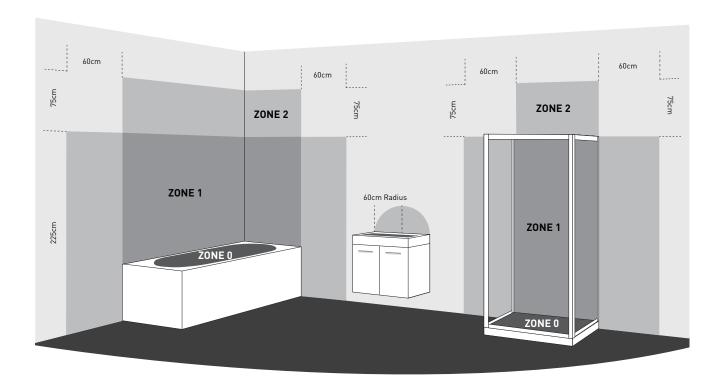
It is important to install light fittings and electric Towel Warmer elements in the correct bathroom zone i.e. the zone referred to in the IP rating of the element. This is not an installation guide and reference should be made to the latest edition of the IET Wiring Regulations or a qualified electrician member of NICEIC or IET.
