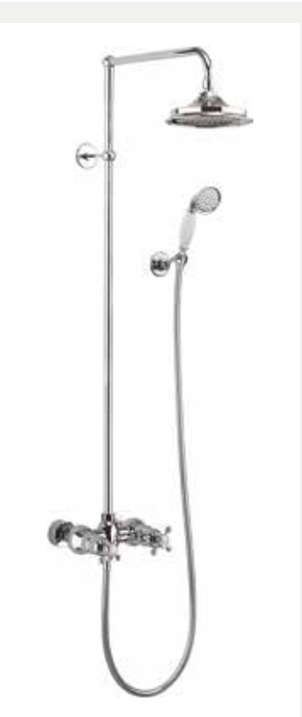
Thermostatic two outlet twin control valve with independent flow diverter and temperature control Traditional brass body and Claremont handle with ceramic indices Adjustable wall bracket, 1500mm shower hose and handset with ceramic handle 18mm diameter vertical brass shower riser 355mm adjustable swivel shower arm 6", 9", 12" AirBurst shower head
